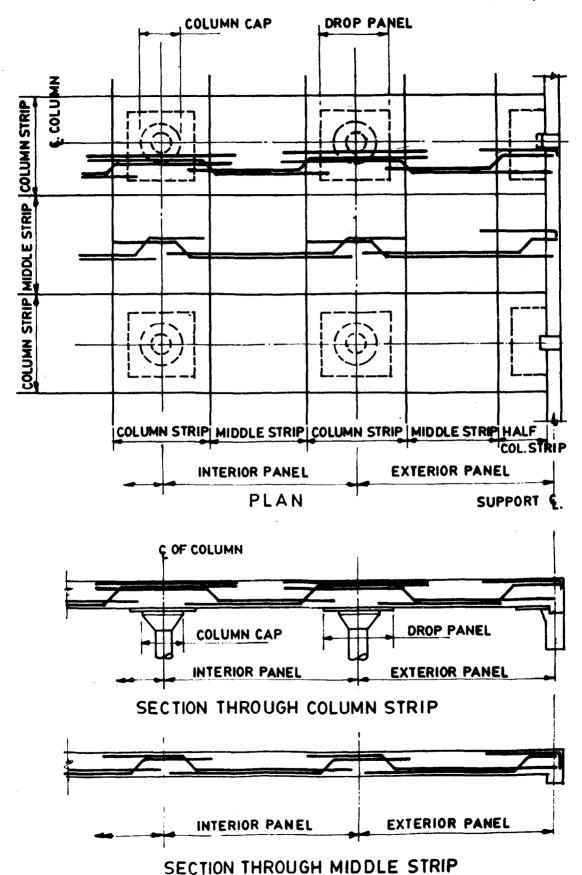
FIG. 9.17 TYPICAL ARRANGEMENT OF BARS IN A FLAT SLAB WITH DROP PANELS
