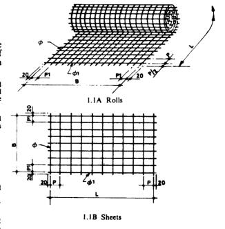
FIG. 1.1 WELDED WIRE FABRIC
