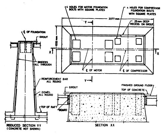
FIG. 11.32 TYPICAL FOUNDATION FOR INSTRUMENT AIR COMPRESSOR
