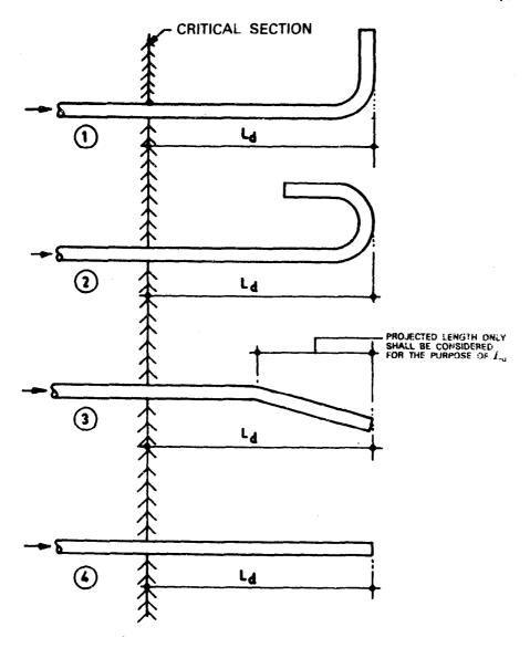
Note — In compression hooks and bends are ineffective and cannot be used as anchorage.
