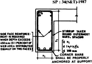
8.14A SHEAR AND TORSION REINFORCEMENT IN BEAMS
