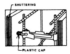
Fig. 13.12 Spacers for Reinforcement and Shuttering
