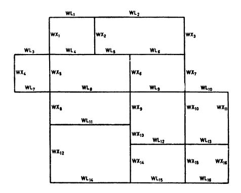
FIG. 3.4 TYPICAL MARKING DETAILS FOR WALLS
