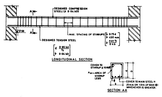
FIG. 8.11 REINFORCEMENT REQUIREMENTS FOR BEAMS
