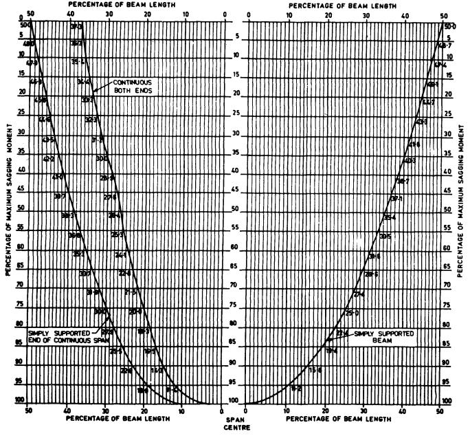
FIG. 4.23 STANDARD BENDING MOMENT DIAGRAMS (BASED ON UDL)
