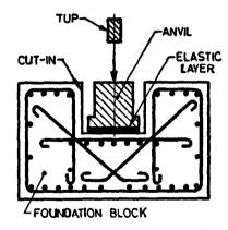
FIG. 11.28 Typical Reinforcement Detail
