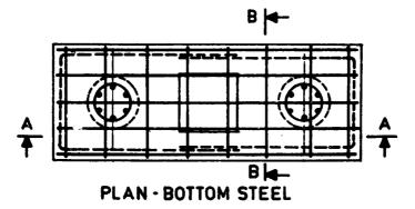
Note—In a 2-pile system, sufficient care should be taken to transfer bending in the transverse direction.
