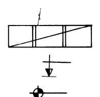
Identical sheets of welded fabric in a row
