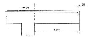
Available space for straight bar = 1400 - 25 = 1375  $L_{\rm d1}$  required (for # 28) = 1580 Straight # 28 will not fit ( $L_{\rm dt} - L_{\rm e}$ ) = 1580 - 224 = 1356  $\therefore \# 28$  Bar with standard bend will fit
