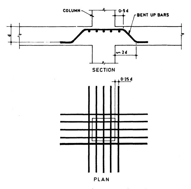
Fig. 9.22 Beam-Cage Stirrups (Supplemented by Bent-up Bars).
