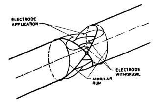
FIG. A-7 MAKING OF TOP BEAD
