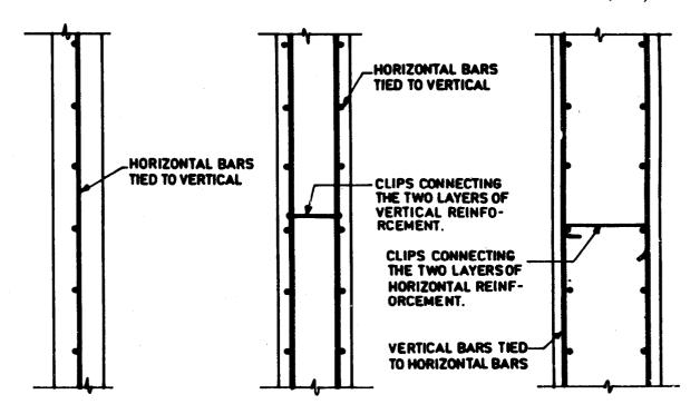
11.6A WALL'S OF THICKNESS ≤ 170 mm. REINFORCEMENT IN CENTRE OF WALL (CONSIDERED TO BE NOMINAL)
