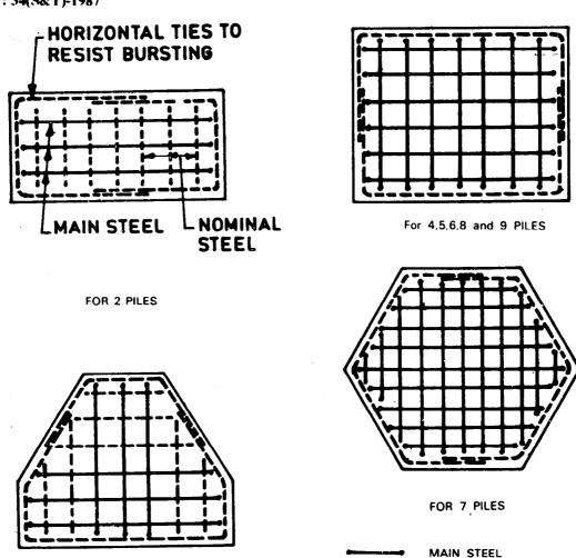
Fig. 6.10 Generally Adopted Configuration for Pile Caps (Along with Plan Arrangement of Reinforcement)
