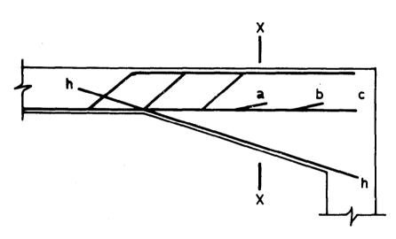
FIG. 8.33 MAIN REINFORCEMENT IN END HAUNCHES (See Fig. 8.33 for Section xx)
