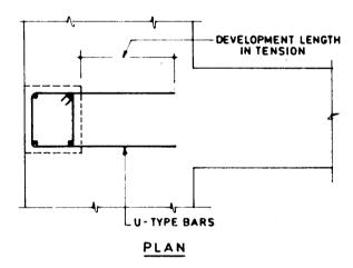
Fig. 6.3 Column on Edge of a Footing
