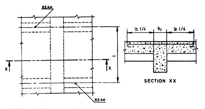
Fig. 8.18 Transverse Reinforcement in Flange of T-Beam when Main Reinforcement of Slab is Parallel to Beam
