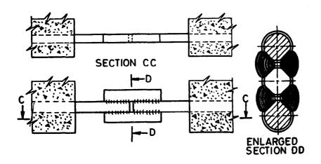
A-2D INDIRECT BUTT SPLICE USING TWO BARS
