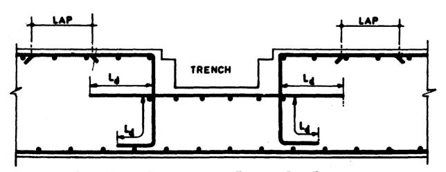
FIG. 6.6 TYPICAL DETAILS AROUND A TRENCH IN RAFT FOUNDATION
