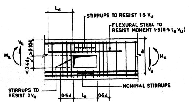
FIG. 8.39 DETAILS OF REQUIREMENTS AT A LARGE OPENING IN THE WEB OF A BEAM
