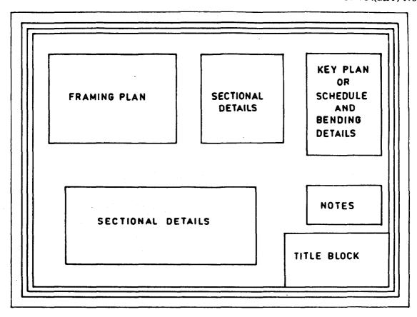
FIG. 3.2 TYPICAL LAYOUT OF A DRAWING
