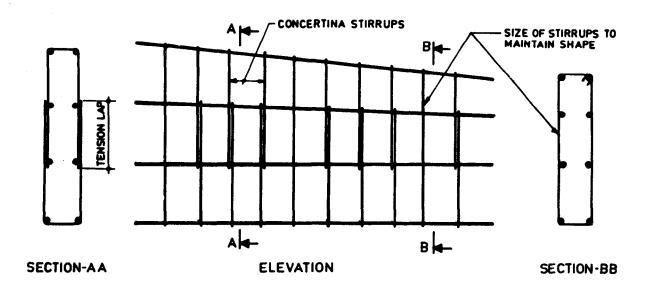
FIG. 8.12 USE OF CONCERTINA STIRRUPS IN BEAMS OF VARYING DEPTH
