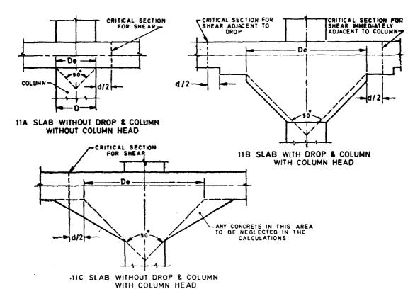
NOTE — De is the diameter of column or column head to be considered for design and d is effective depth of slab or drop as appropriate.
