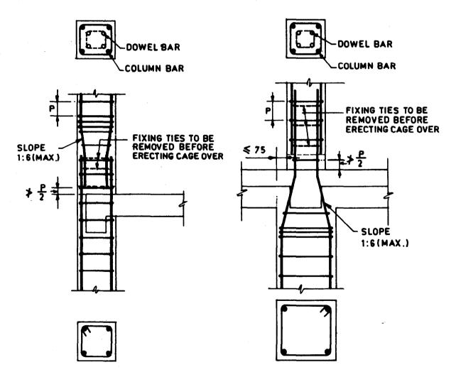
7.9C SPLICE WITH UPPER BARS CRANKED INTO POSITION INSIDE LOWER BARS
