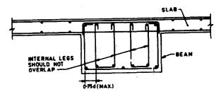
Fig. 8.9 Multi-Legged Open Type Stirrups Cross-Section of a Broad Shallow BEAM WITH 6-LEGGED STIRRUPS
