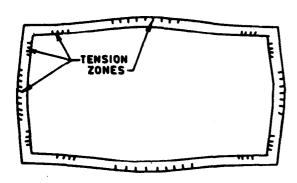
Fig. 11.19 Sketch Showing Deformation of Rectangulor Tank Under Internal Pressure
