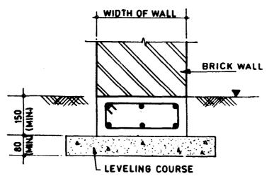
6.14A BEAMS IN NON-EXPANSIVE SOILS
