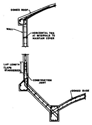
Fig. 11.24 Typical Arrangement of Bars in a Intze Tank
