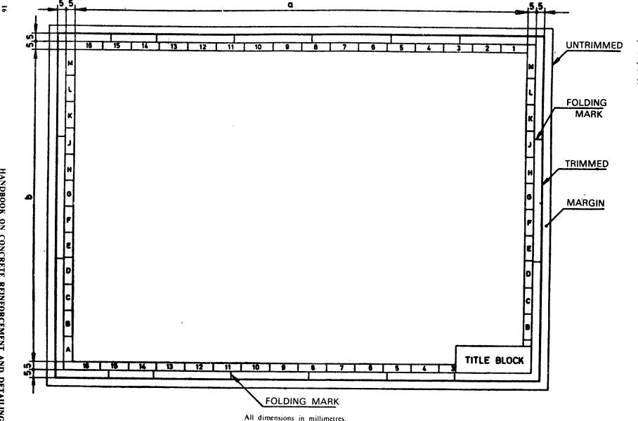
All dimensions in millimetres. 3.1A AO SHEET LAYOUT
