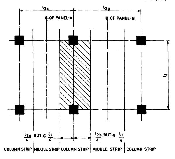
FIG. 9.15 PANELS, COLUMN STRIPS AND MIDDLE STRIPS
