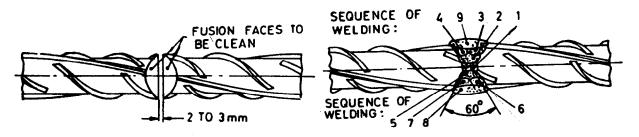
FIG. A-6 SEQUENCE OF WELDING BEADS
