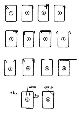
NOTE Preferred shapes for torsion-1,2,3,4,6,7,13 and 14 FIG. 8.6 DIFFERENT SHAPES OF STIRRUPS
