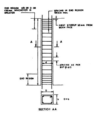
FIG. 12.5 SPACING OF SHEAR REINFORCEMENT IN COLUMNS
