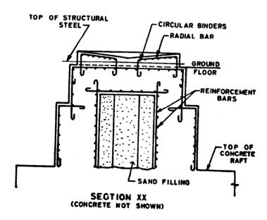
FIG. 11.30 TYPICAL FOUNDATION FOR CRUSTING MILL (PULVERIZER UNIT)
