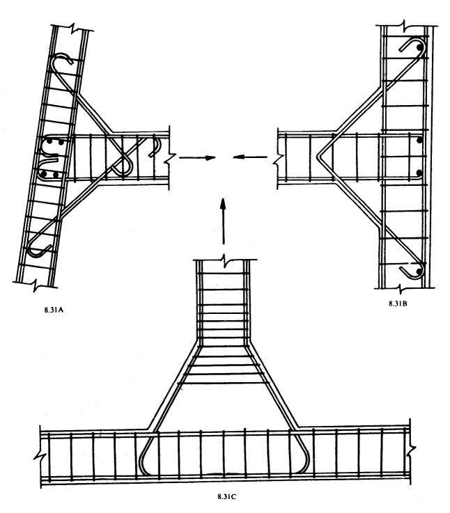
FIG. 8.31 TIE END CONNECTIONS FOR HIGH LOADING
