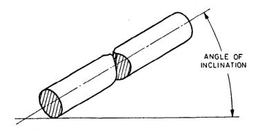
FIG. A-1 EDGE PREPARATION OF INCLINED BARS
