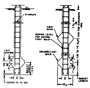
3A SECTION OF SINGLE 3B SECTION OF MULTI UNDER-REAMED PILE. UNDER-REAMED PILE.
