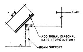
FIG. 9.6 ADDITIONAL REINFORCEMENT AT RE-ENTRANT CORNERS
