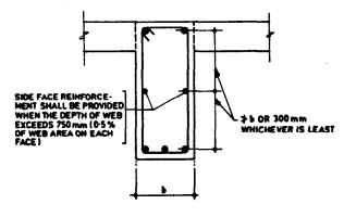
FIG. 8.4 SIDE FACE REINFORCEMENT IN BEAMS
