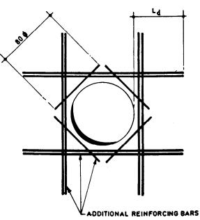
FIG. 9.11 ADDITIONAL REINFORCEMENT AROUND A CIRCULOR OPENING IN A SLAB
