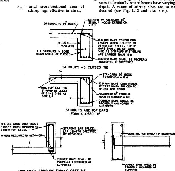
FIG. 8.10 TYPICAL DETAILS OF REINFORCEMENT IN EDGE AND SPANDREL BEAM
