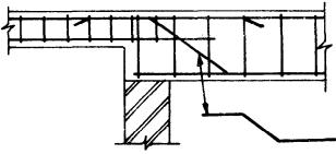
Fig. 8.29 Beams at Different Depths
