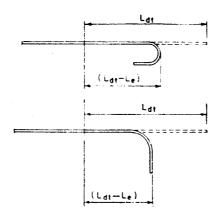
When hooks/bends do not conform to standard bends/hooks given in Table 4.1, anchorage value of hook/bend shall be neglected and the total development length provided (measured along bend/hook) shall be equal to the required development length ( $L_{\rm dt}$ ).
