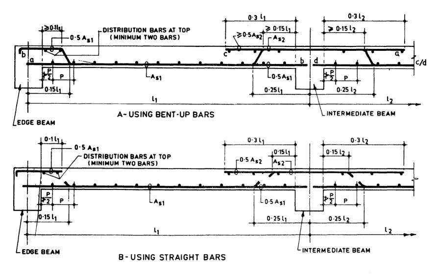
FIG. 9.5 SIMPLIFIED RULES FOR CURTAILMENT OF BARS-SECTION THROUGH MIDDLE STRIP
