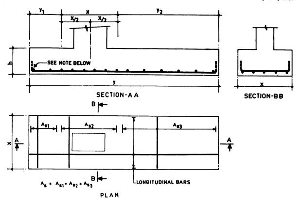
Note — Provide standard 90° bend, if the bar is required to be bent upwards to get required development length.
