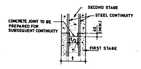
Fig. 11.18A A Construction Joint
