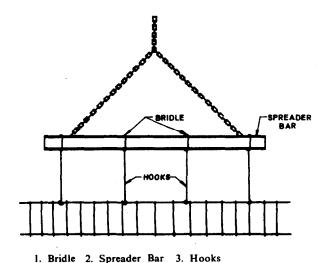
FIG. 13.5 HOISTING EQUIPMENT
