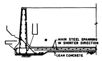
Fig. 11.21 Rectangular Tank Restrained at Base with Thickening at the base— Typical Cross Section
