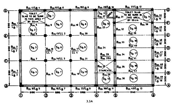
Fig. 3.3 Typical Arrangement for the Key Framing Plan and Marking Different Structural Members (Continued)
