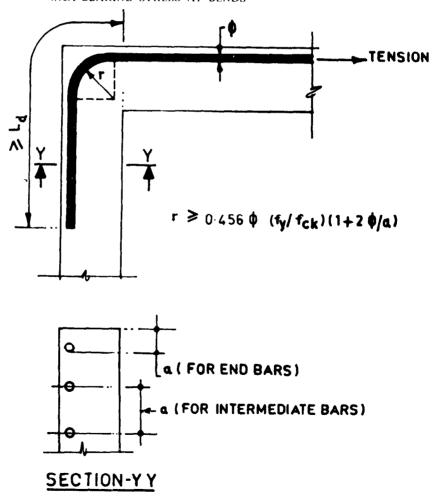
4.16B MINIMUM INTERNAL RADIUS OF BEND FOR EFFECTIVE ANCHORAGE OF FULLY STRESSED TENSION BARS
