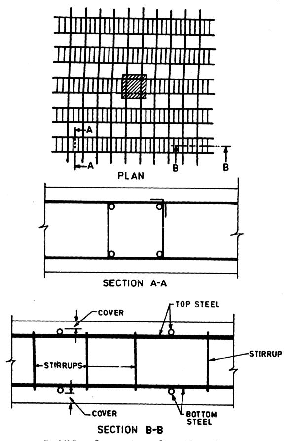
Fig. 9.18 Shear Reinforcement for Slab at Column Heads
