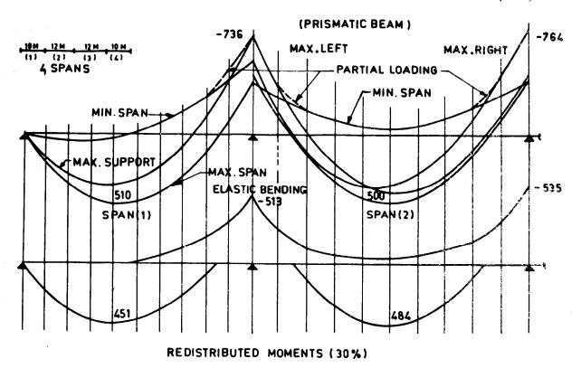
FIG. 4.22 A TYPICAL BENDING MOMENT ENVELOPE
