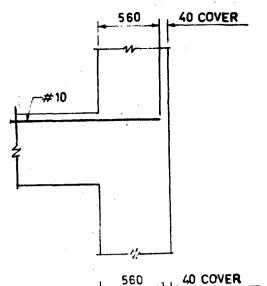
Available space for straight bar = 560  $I_{\rm dt}$  required ( for #10 ) = 564  $\therefore$  Straight bar # 10 will fit
