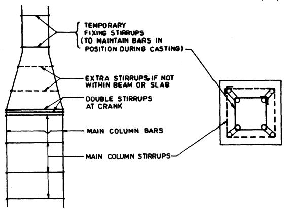
FIG. 7.7 TEMPORARY FIXING OF STIRRUPS
