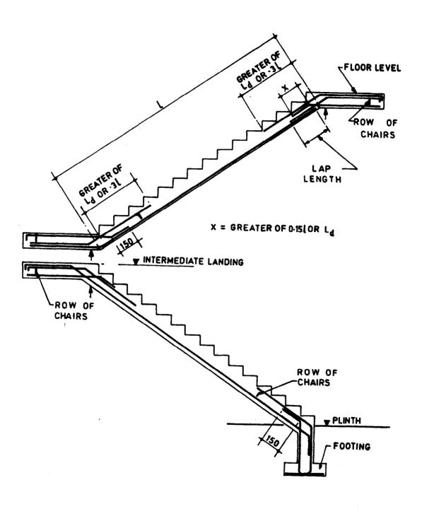
FIG. 10.4 STAIRS SUPPORTED AT ENDS OF FLIGHTS-SHOWING MAIN REINFORCEMENT
