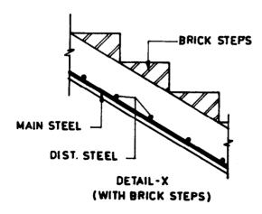
FIG. 10.3 STAIRS SUPPORTED AT ENDS OF LANDINGS—SHOWING POSITION OF MAIN REINFORCEMENT
