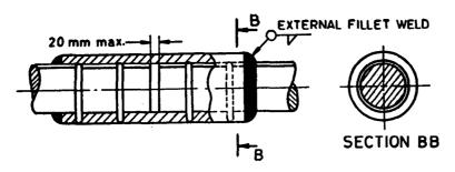
A-2C INDIRECT BUTT SPLICE USING A SLEEVE
