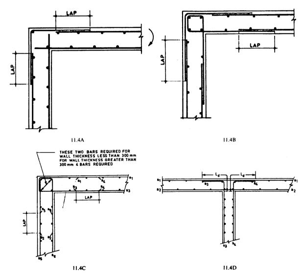
FIG. 11.4 TYPICAL CORNER AND INTERSECTION DETAILS FOR REINFORCED CONCRETE WALLS
