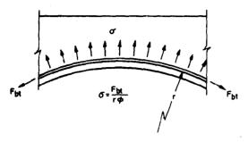
4.17A TENSION BAR IN A CURVED SOFFIT
