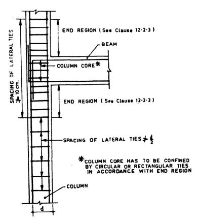
FIG. 12.4 BEAM COLUMN JOINT AT EXTERNAL COLUMNS
