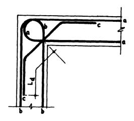
FIG. 8.22 HAIRPIN WITH SPLAY REINFORCEMENT
