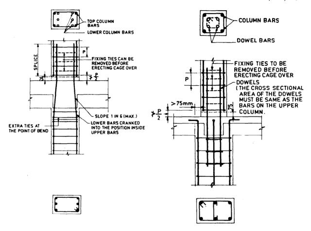
7.9A SPLICE WITH LOWER BARS CRANKED INTO POSITION INSIDE UPPER BARS (INTERMEDIATE FLOOR)
