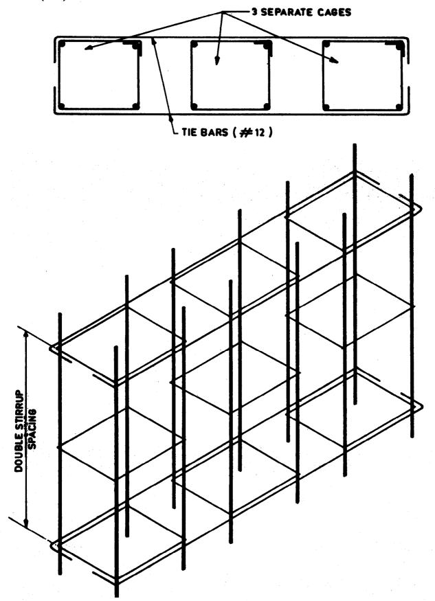
FIG. 7.8 REINFORCEMENT IN CAGES FOR LONG COLUMNS
