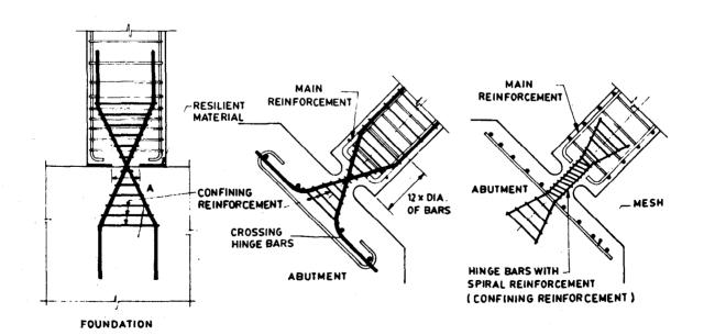
FIG. 11.25 REINFORCED CONCRETE HINGES AT SUPPORTS
