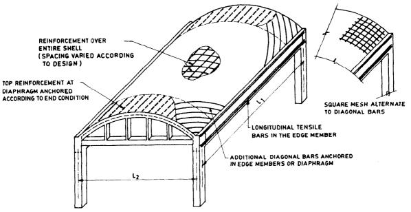
H.14A ISO METRIC VIEW OF A BARREL SHELL
