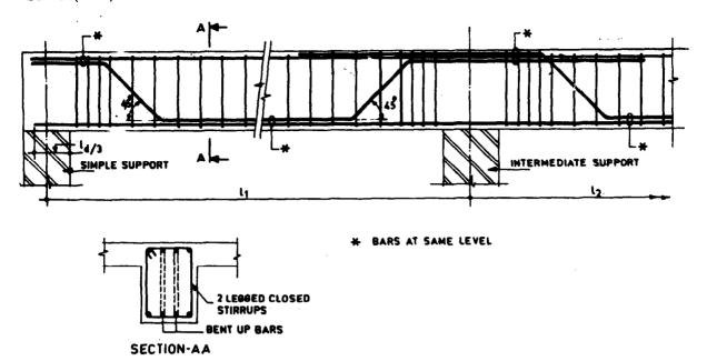
8.7B TYPICAL ARRANGEMENT OF BENT-UP BARS AND VERTICAL STIRRUPS IN A CONTINUOUS BEAM FIG. 8.7 BENT-UP BARS
