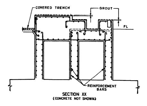
FIG. 11.31 TYPICAL FOUNDATION FOR PRINARY AIR FAN
