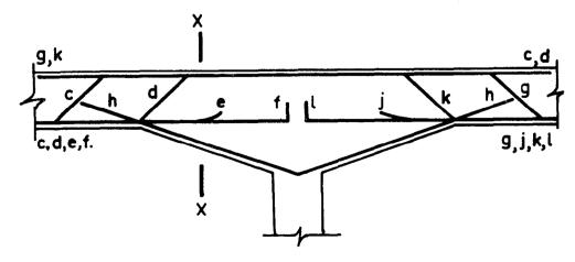
FIG. 8.34 MAIN REINFORCEMENT IN HAUNCHES (See Fig. 8.37 FOR SECTION XX)
