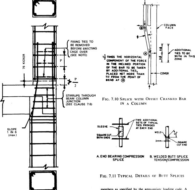
7.9E Splicing when the Lower Bars Cranked into a Position inside the Upper Bars with Stepping of Columns on One Side
