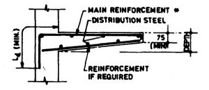
50 % OF MAIN REINFORCEMENT CAN BE CURTAILED AT A DISTANCE OF 0-5 L OR L4 FROM THE FACE OF SUPPORT
