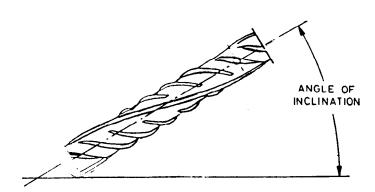
FIG. A-5 EDGE PREPARATION OF INCLINED BARS
