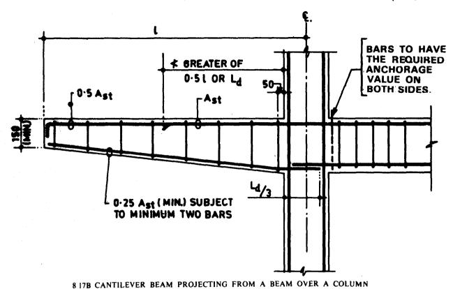
FIG. 8.17 SIMPLIFIED CURTAILMENT RULES FOR A CANTILEVER BEAM
