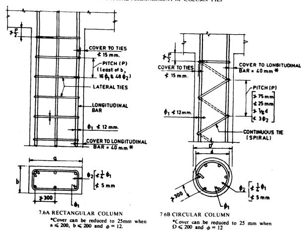
FIG. 7.6 BAR SPACING REQUIREMENTS IN COLUMNS
