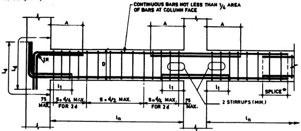
Designer should provide dimension A, S, d, anchorage length, cutoff points of discontinuous bars, etc. \*provide not less than two stirrups throughout splice length.  $A = \text{distance to point of inflection plus anchorage length but not less than } l_n/4$ . Designer may cut some
