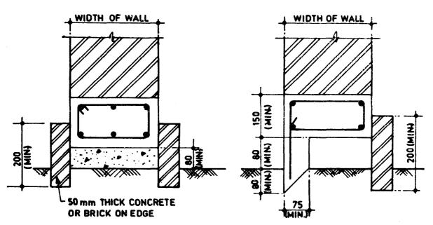
6.14B BEAMS IN EXPANSIVE SOILS Fig. 6.14 Typical Sections of Grade Beams
