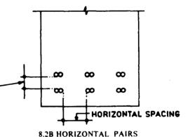
VERTICAL SPACING SHOULD BE NOT LESS THAN 15 m m OR 2/3 ha OR • WHICHEVER IS GREATER.
