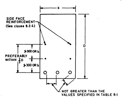
FIG. 8.3 REINFORCEMENT SPACING RULES FOR CRACK CONTROL
