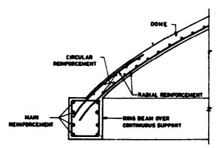
FIG. 11.16 REINFORCEMENT IN A DOME
