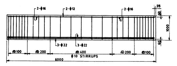
SECTIONAL ELEVATION OF DIAPHRAGM
