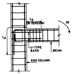
TROOF LEVEL FIG. 7.15 TYPICAL DETAILS OF A BEAM-COLUMN JUNCTION AT EXTERIOR COLUMN
