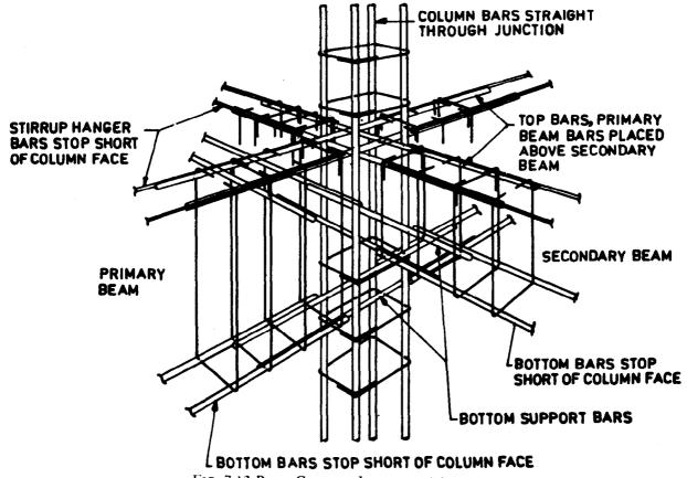
FIG. 7.13 BEAM-COLUMN INTERSECTION
