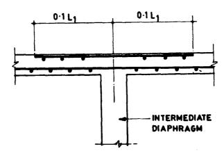
11.14C REINFORCEMENT NEAR AN INTERMEDIATE DIAPHRAGM.
