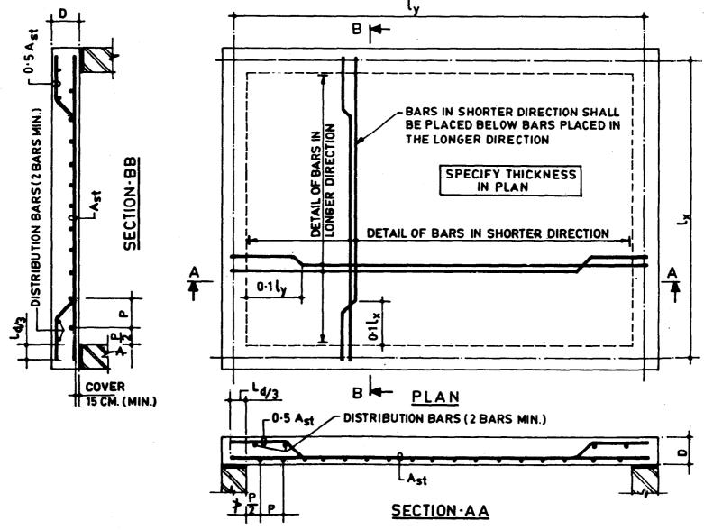
FIG. 9.2 TYPICAL DETAILS OF A SLAB SPANNING IN TWO DIRECTIONS
