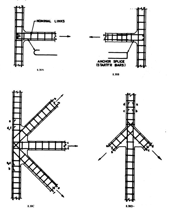
FIG. 8.30 TIE END CONNECTIONS FOR LIGHT LOADING
