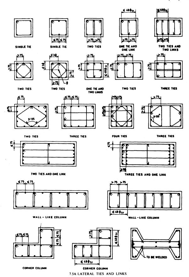
FIG. 7.5 TYPICAL ARRANGEMENT OF COLUMN TIES (Continued)
