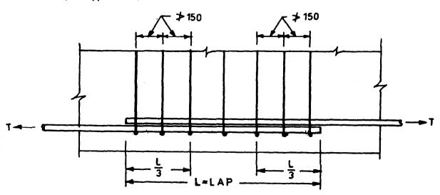
FIG. 4.3 TRANSVERSE REINFORCEMENT AT A SPLICE
