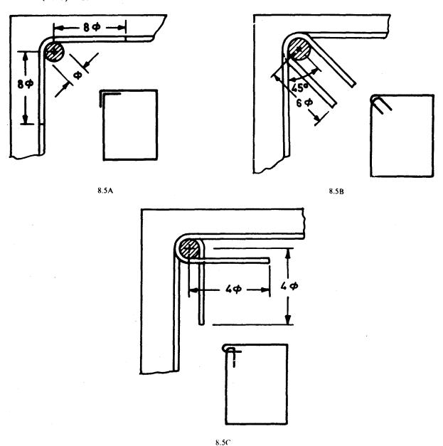
Fig. 8.5 Different Ways of Anchoring Ends of Stirrups
