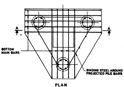
FIG. 6.12 TYPICAL DETAILS OF A 3-PILE CAP
