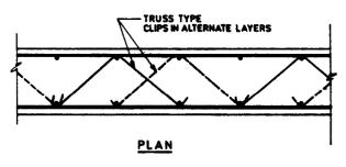
Fig. 11.7 Truss-Type Clips in Alternate Layers in a Wall
