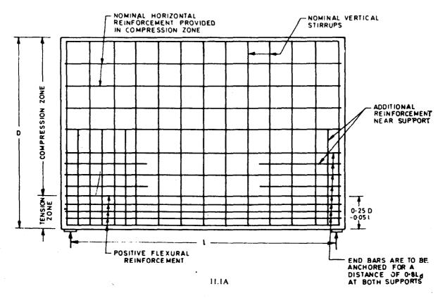
FIG. 11.1 REINFORCEMENT DETAILING IN SIMPLY SUPPORTED DEEP BEAMS (Continued)
