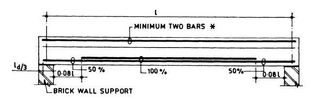
\*In case partially restraint members, 35 percent of the reinforcement shall also be provided for negative moment at the support and fully anchored.
