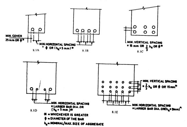
FIG. 8.1 MINIMUM CLEARANCE BETWEEN INDIVIDUAL BARS
