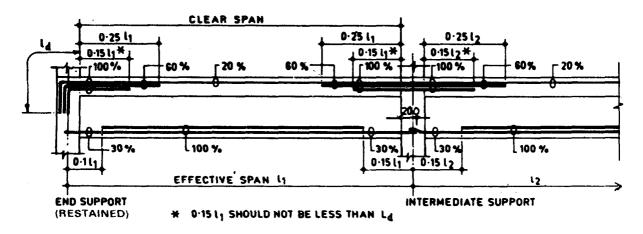
NOTE Applicable to continuous beams with approximately equal spans (not differing more than 15 percent) and subjected to predominantly U.D.L., and designed without compression steel.
