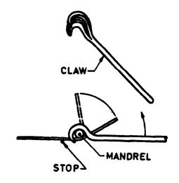
FIG. 13.1 BENDING OF BAR BY MEANS OF CLAW
