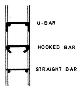
FIG. 13.11 SPACERS FOR VERTICAL LAYERS
