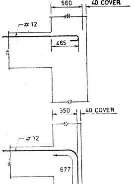
Available space for straight bar = 560  $L_{\rm dt} \text{ required ( for } \# 12 \text{ )} = 677$ Straight bar will not fit  $(L_{\rm dt} - L_{\rm e}) = (677 - 192) = 485$   $\therefore \# 12 \text{ with standard hook will easily fit}$
