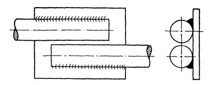
A-3B LAP WELDING BARS WITH BARS SEPARATED BY A DISTANCE
