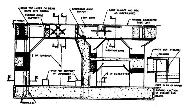
11.33A TYPICAL LONGITUDINAL SECTION THROUGH A TURBO GENERATOR FOUNDATION FIG. 11.33 TYPICAL DETAILS OF A TURBO GENERATOR FOUNDATION (Continuted)
