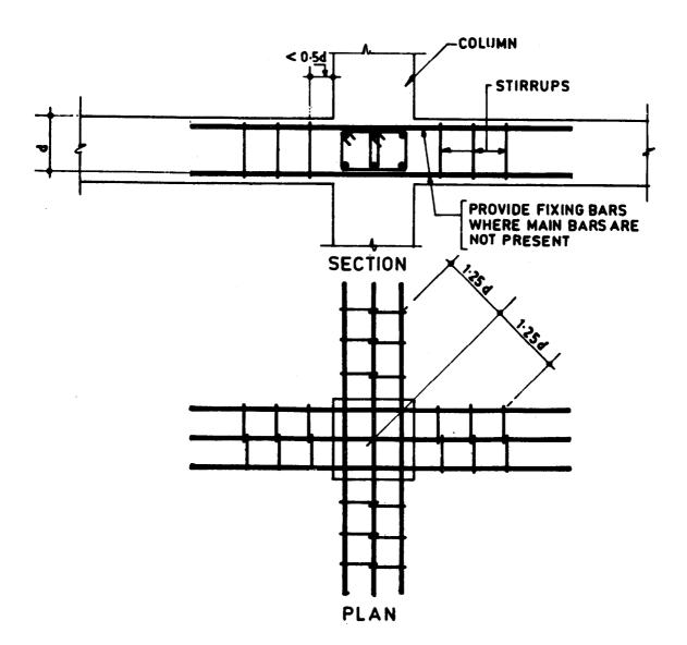
FIG. 9.21 BEAM-CAGE STIRUPPS (SUPPLEMENTED BY ISOLATED STIRRUPS).
