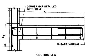
FIG. 10.8 TYPICAL DETAILS OF A STAIR CASE CANTILEVERING FROM THE SIDE OF A WALL
