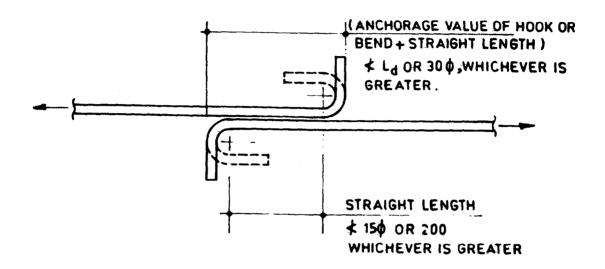
.N FLEXURAL TENSION WITH HOOKS
