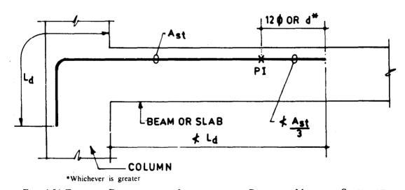
FIG. 4.21 TENSILE DEVELOPMENT LENGTHS FOR POSITIVE MOMENT STEEL AT DISCONTINUOUS ENDS
