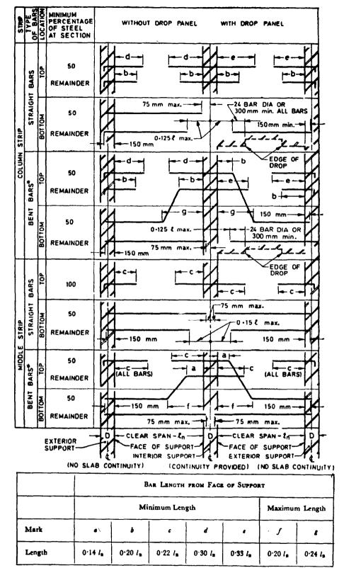
Bent bars at exterior supports may be used if a general analysis is made.
