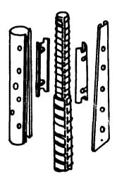
FIG. 4.15 COUPLING WITH SLEEVE AND WEDGE
