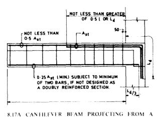
Fig. 8.17 Simplified Curtailment Rules for a Cantilever Beam (Continued)
