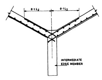
11.14B REINFORCEMENT NEAR AN INTERMEDIATE EDGE MEMBER
