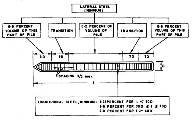
Fig. 6.7 Minimum Steel Requirements of Precast Concrete Pile
