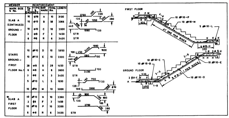
Fig. 10.10 AN Example of a Stair with Placing Detail and Bending Schedule
