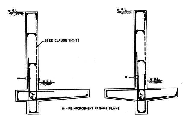
Fig. 11.9 L-Walls (Distribution Bars Omitted for Clarity)
