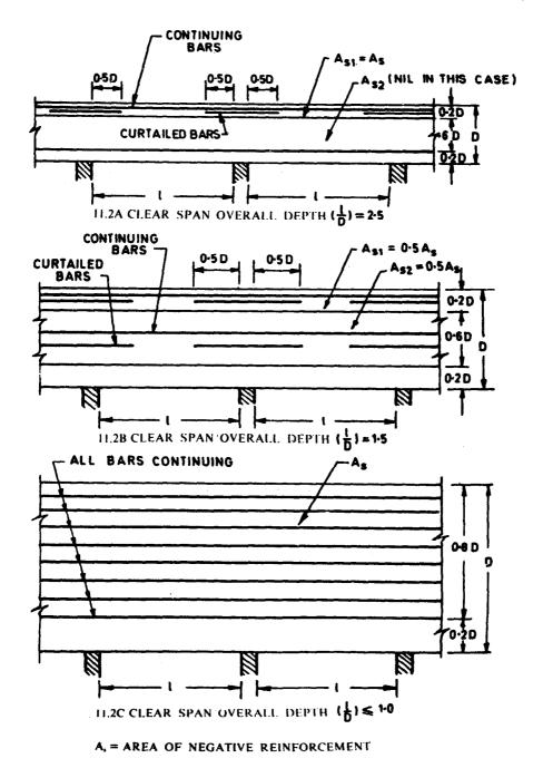
FIG. 11.2 DISPOSITION OF NEGATIVE REINFORCEMENT IN CONTINUOUS DEEP BEAMS
