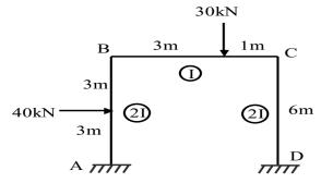
Using the strain energy method find forces the **member AD** of truss loaded as shown in fig.
