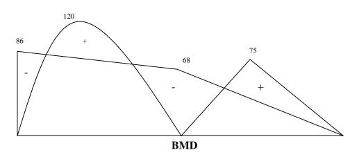
2. Analyse the continuous beam shown in the figure by flexibility matrix method, draw BMD
