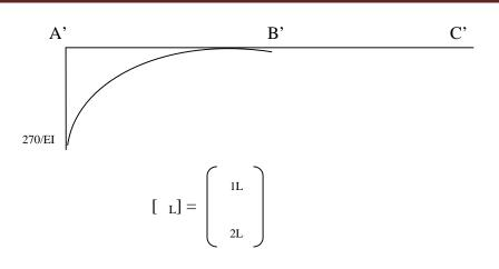
$_{1L}$  = Displacement at B in primary determinate structure = BM at B' in conjugate beam
